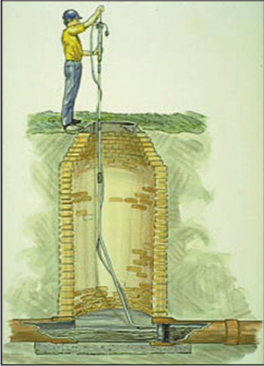
Figure 1: Flow mapping using a flow meter.
