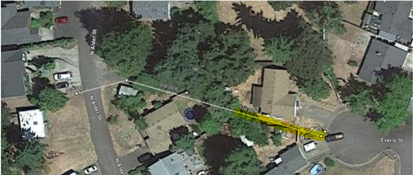
Figure 3: Storm Line (Approximate Location) CCTV Surveyed
