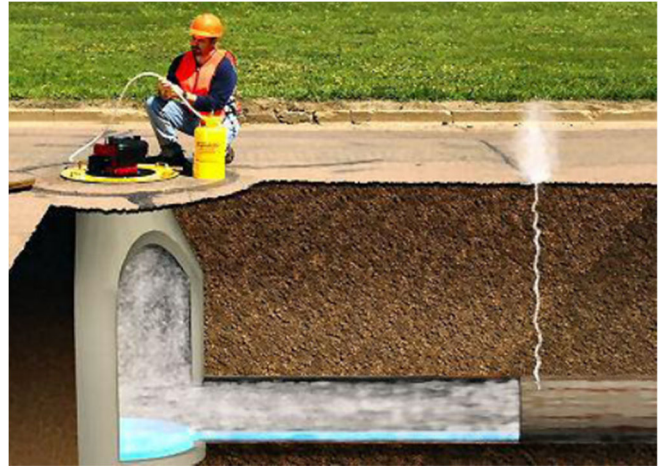
Figure 2: Smoke testing the sanitary sewer system to identify inflow sources.
