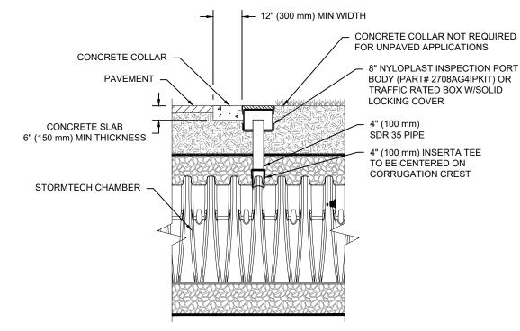
INSPECTION PORTS MAY BE CONNECTED THROUGH ANY CHAMBER CORRUGATION CREST.
