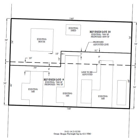
Figure 1. Proposed Property Line Adjustment Site Plan.
